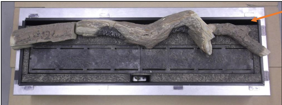
Rear warm air outlet slot Lay 3 back logs as shown and note that only the curved section on the centre log is permitted to cover the rear warm air outlet slot which has been sized to allow for this.
