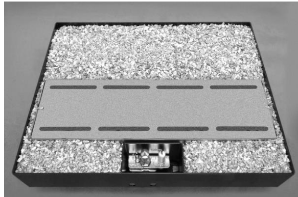
Typical burner showing beige insulation pad in position and vermiculite fill, ready to lay ceramics. The pilot cut-out is normally in the centre at the front. As an alternative a side pilot cut-out is sometimes supplied.
